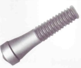
GINA - A round finger with a special profile, especially fits STORK and MEYN pickers. The combination of a round and gentle finger profile with a special rib design gives this finger excellent picking capacity. The shape of the finger's head and neck gives it a strong and stable hold in the disc and therefore it is also longer lasting. GINA fingers are produced in a wide range of hardness degrees to fit all requirements, from very soft M-45 compound to very hard M-140.
